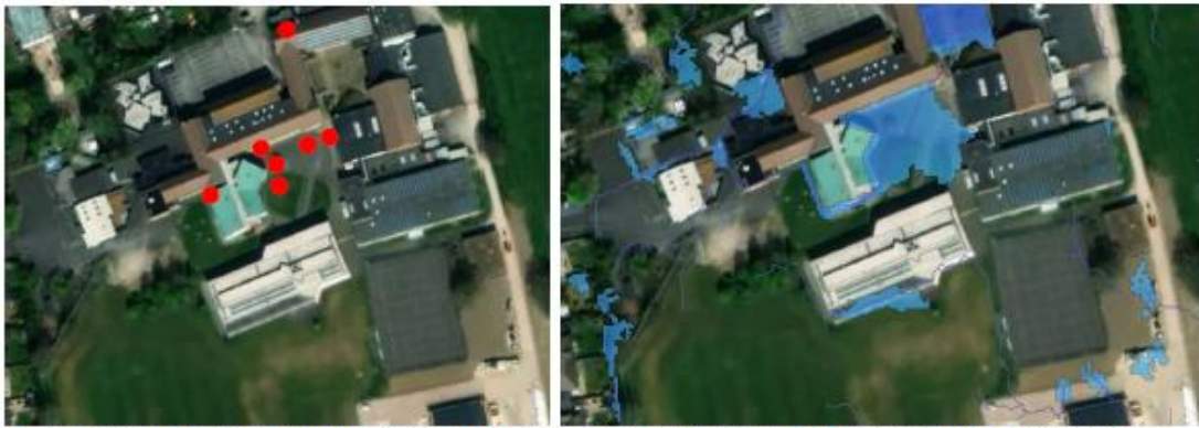
Fig. 2: Location of 7 rain-planters installed by OART & surface water pathways at Kings Academy (Scalco 40mm rainfall)
